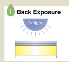
Expose to UV light through substrate film on back side of plate.
