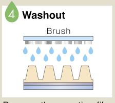
Remove the negative film and process the plate in Cosmolight® washout unit.
