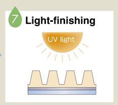
Expose to UV-C light to eliminate the tackiness of the plate surface.
