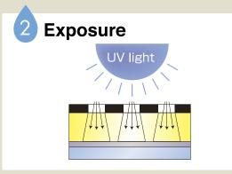
Expose the plate through the negative film to UV light having 360 nm wave length. Determine the correct exposure time using a 21 steps grey scale. Follow "TIPS FOR Printight®" in each case.
