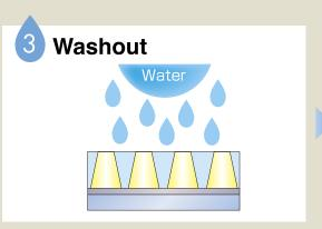
Remove the negative film. Washout the exposed plate with water. Use the special washout machine suitable for TOYOBO Printight®. Washout time depends on the thickness of the plate. Follow "TIPS FOR Printight®" in each case. Rinse the washed out plate with fresh water.
