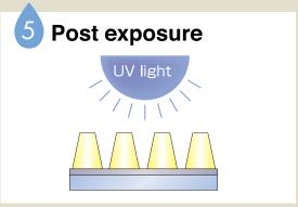
Expose the developed plate after drying again to UV light in order to get stability. Post exposure time should be the same or longer than main exposute time.
