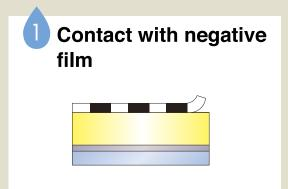
Remove the cover film and place a negative film on the undeveloped plate. Use a negative film having the optical density of no less than 3.0.
