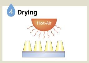
Dry the plate in a hot-air dryer after takingoff the surface water with a sponge roll. Drying time depends on the type of the plate. Follow "TIPS FOR Printight®" in each case.
